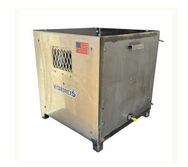
The Hydrorex Model PTC-24 Burst and Hydrostatic Test Chamber is a high-performance enclosure bunker for destructive and non-destructive testing applications... Manufactured and designed for high pressure resistance up to 60,000 psi per API requirements... All Stainless steel walls reinforced with wood to cushion the impact.
