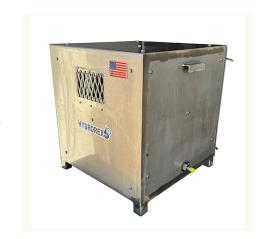
The Hydrorex Model PTC-16 Burst and Hydrostatic Test Chamber is a high-performance enclosure bunker for destructive and non-destructive testing applications... Manufactured and designed for high pressure resistance up to 60,000 psi per API requirements... All Stainless steel walls reinforced with wood to cushion the impact.
