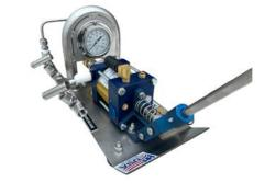
The HIP series pump is self priming for immediate operation. Hand pump attachment allows for manual operation when shop air is not available or for **Precision Pressure Control**. Safe, durabble and easy to operate. Made in USA with highest quality components. Available for use on a wide range of fluids including water, oil/hydraulic and other solubles; **Designed** for Hydrostatic, Calibration, Pressure Certification, Burst, Booster, Hydro, Injection, Leak Detector, and More.
