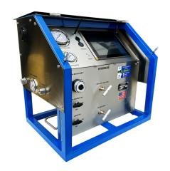
Digital hydrostatic pressure test unit is the most common standard testing equipment with digital pressure and temperature graph chart recorder with a 0.15% accuracy. Air operated liquid pressure pump with a variety of models on pressure that ranges from 500 PSI to 65,000 PSI, with several flow rates.
