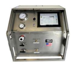
Digital hydrostatic pressure test unit is the most common standard testing equipment with digital pressure and temperature graph chart recorder with a 0.15% accuracy. Air operated liquid pressure pump with a variety of models on pressure that ranges from 500 PSI to 65,000 PSI, with several flow rates.
