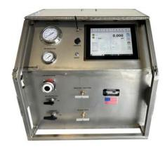
Digitial hydrostatic pressure test unit is the most common standard testing equipment with digital pressure and temperature graph chart recorder with a 0.15% accuracy. Air operated liquid pressure pump with a variety of models on pressure that ranges from 500 PSI to 65,000 PSI, with several flow rates.
