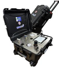
Pressure System with Digital Chart Recorder with a 0.15% accuracy in multiple pressure ranges with customizable test reports in a lightweight yet rugged mobile weatherproof case. Easy Software Interface for Real-Time Pressure, Temperature Monitoring, Reporting and record pressure. Light Weight Design (65 lbs.)
