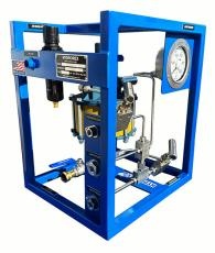
Air operated liquid system that is lightweight portable, economic, safe, durable and easy to operate. Made in USA with highest quality components for low operational cost. Available for use on a wide range of fluids including water, oil/hydraulic and other solubles; requires 80-100 psi air drive pressure to operate. **Designed for Hydrostatic, Burst, Booster, Hydro, Injection, Leak Detector, Pressure Calibration and More**.
