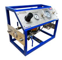
Air operated liquid system that is lightweight portable, economic, safe, durable and easy to operate. Made in USA with highest quality components for low operational cost. Available for use on a wide range of fluids including water, oil/hydraulic and other solubles; requires 80-100 psi air drive pressure to operate. **Designed for Hydrostatic, Burst, Booster, Hydro, Injection, Leak Detector, Pressure Calibration and More**.
